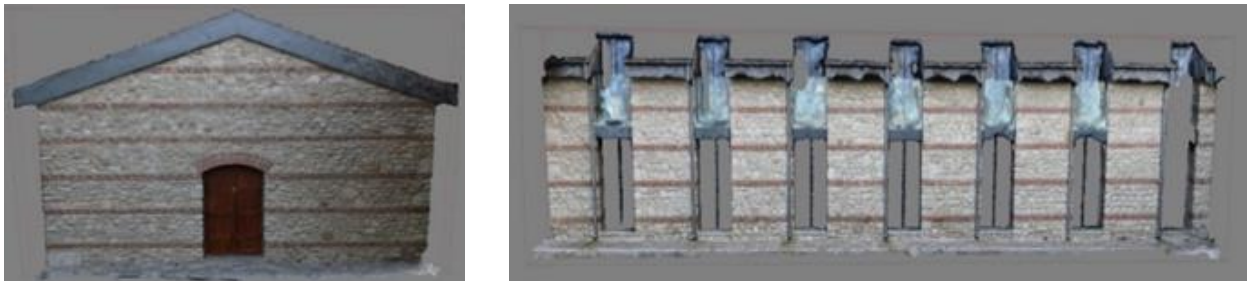
Figure 2. The point cloud models of two different facades of the guesthouse
