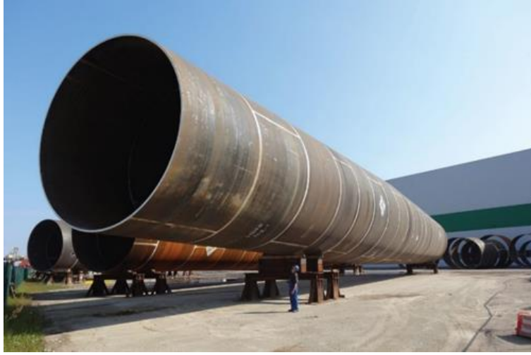
Figure 1. A 7.5 m diameter monopile for Gode Wind Offshore Wind Farm [3]
