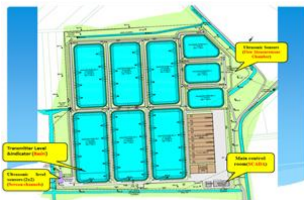
Figure 5. Position of instruments for control and monitoring
