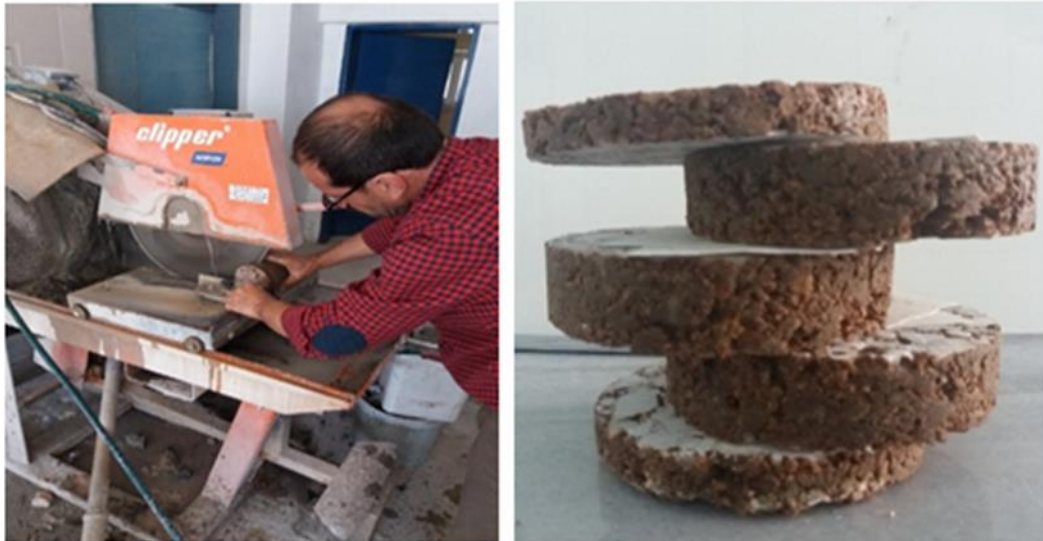
Figure 4. Cutting of the specimens and the resulting horizontal sections.
