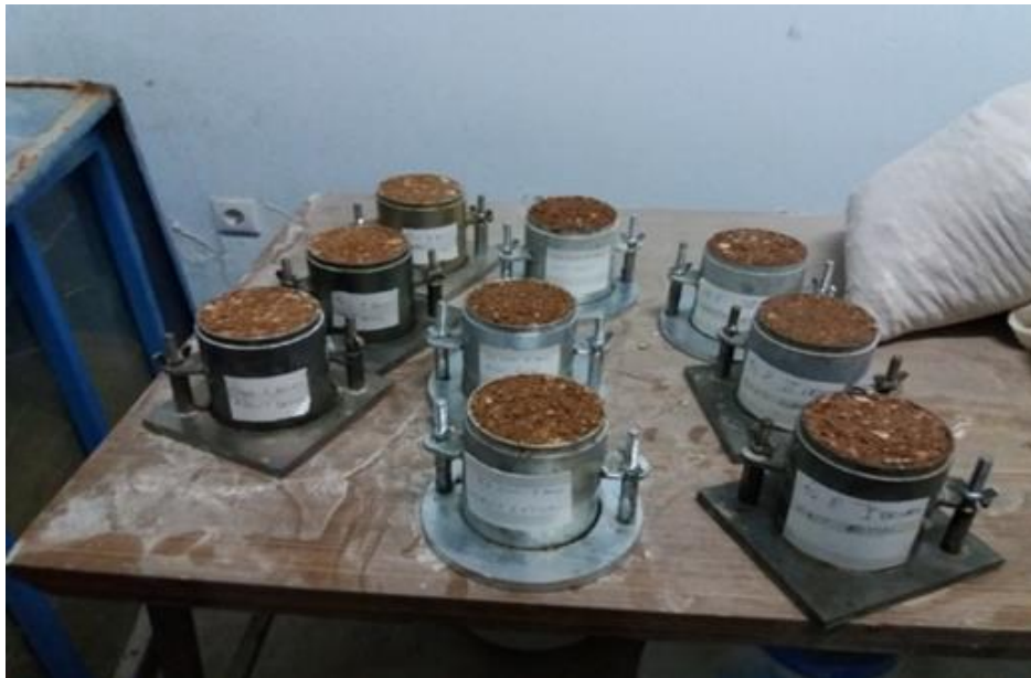
Figure 3. Specimens prepared with epoxy.
