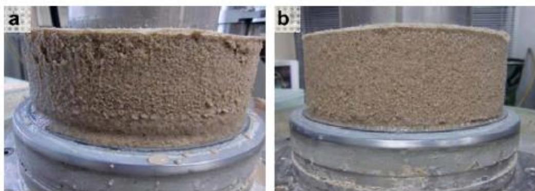
**Figure 4.** Liquefied dense samples after shearing: (a) Sand; (b) fiber 0.4% [6].
