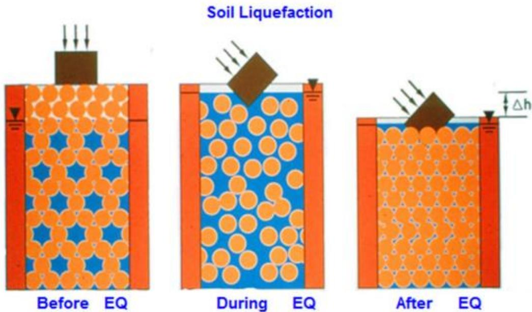
Figure 1. Liquefaction scheme [3]
