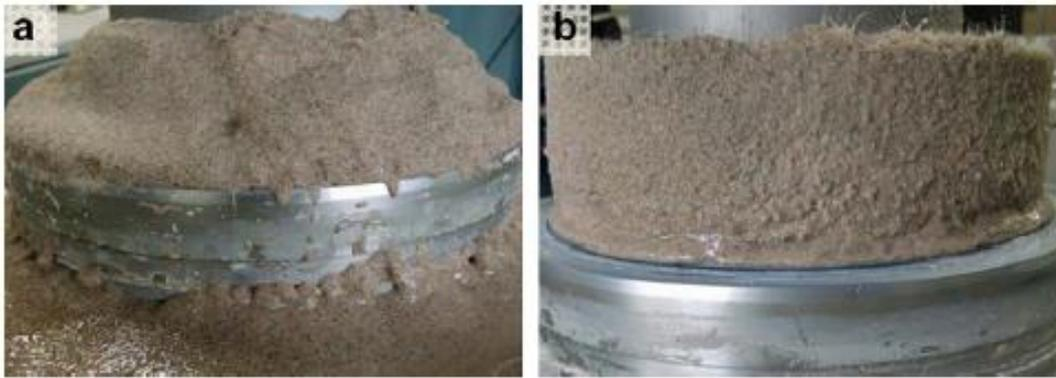
**Figure 2.** Liquefied loose specimens after shearing: (a) Sand; (b) fiber 0.4% [6].
