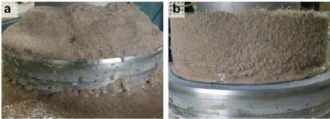
Figure 2. Liquefied loose specimens after shearing: (a) Sand; (b) fiber 0.4% [6].
