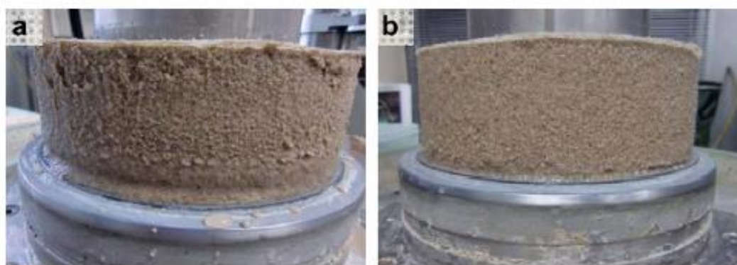
Figure 4. Liquefied dense samples after shearing: (a) Sand; (b) fiber 0.4% [6].
