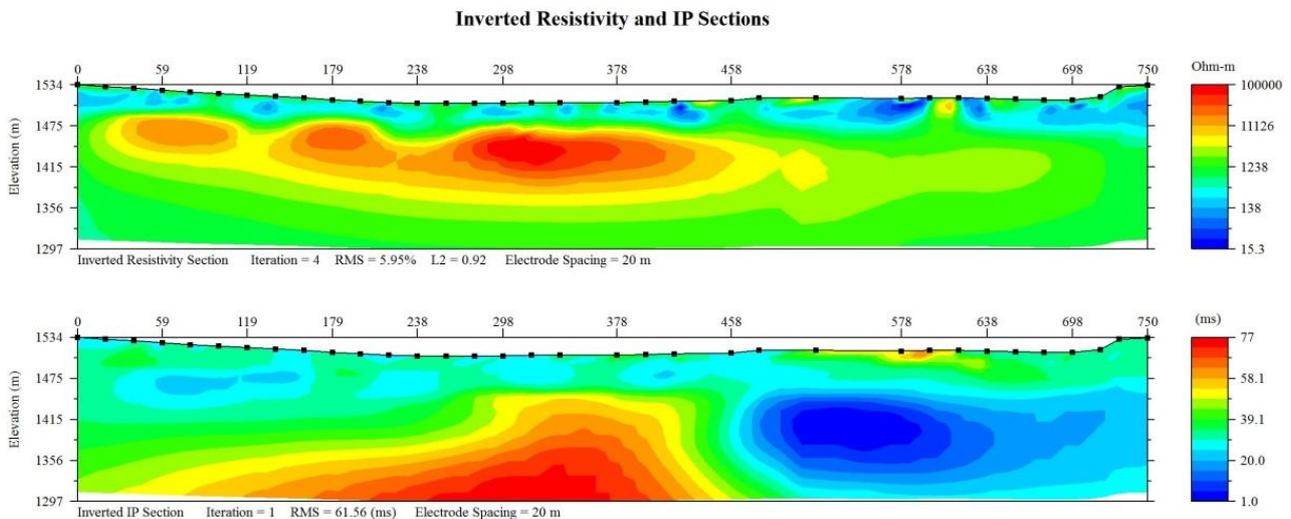
**Figure 1.** The inverted resistivity and IP sections of the 1<sup>st</sup> profile.
