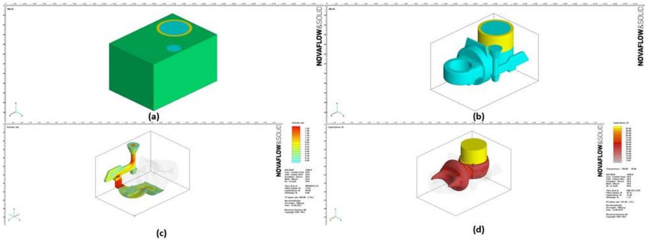
**Figure 4.** (a); The image of the molding design of the casting part, (b); The image of the casting part geometry, (c); The image of the metal flow and filling simulation of the casting part, (d); The image of the friction liquid mod of the casting part
