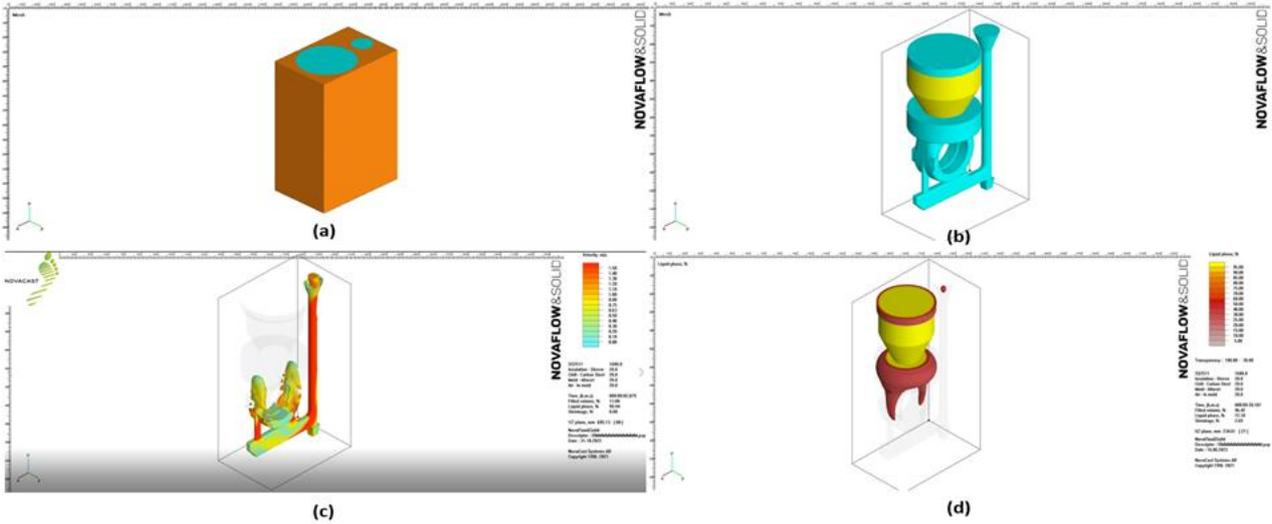
**Figure 2. (a);** The image of the molding design of the casting part, **(b);** The image of the casting part geometry, **(c);** The image of the metal flow and filling simulation of the casting part, **(d);** The image of the friction liquid mod of the casting part
