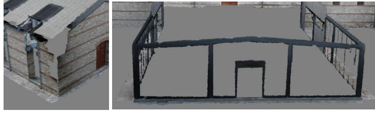
Figure 4. Point cloud loss due to trees and glass-fronted facades
