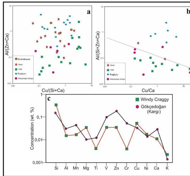
**Figure 2.** a) Al/(Zn+Ca) vs. Cu/(Si+Ca) diagram, b) Al/(Si+Ca+Zn) vs. Cu/Ca diagram, c) Spider diagram for Besshi Type deposits.
