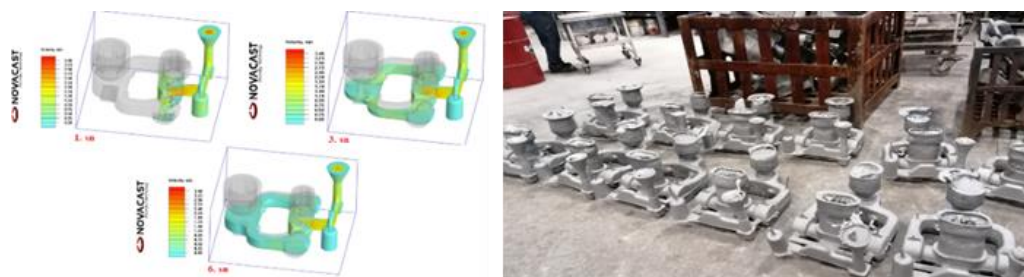
Figure 2. Image of the metal flow and filling simulation and the pouring parts with Spin Trap chamber
