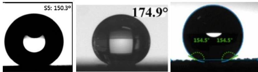
Figure 3. Contact angle images and results [20,21,30]
