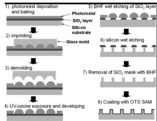
**Figure 2.** Schematic of fabrication process (lithography), [22]
