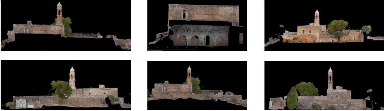
Figure 1. Obtaining the scaled orthophotographs of the building in the programme named PointCab Origins 4
