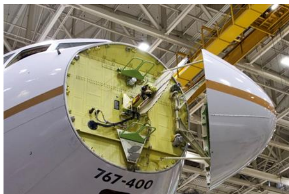
Figure 1. Representation of the radom in the nose of the aircraft [2]
