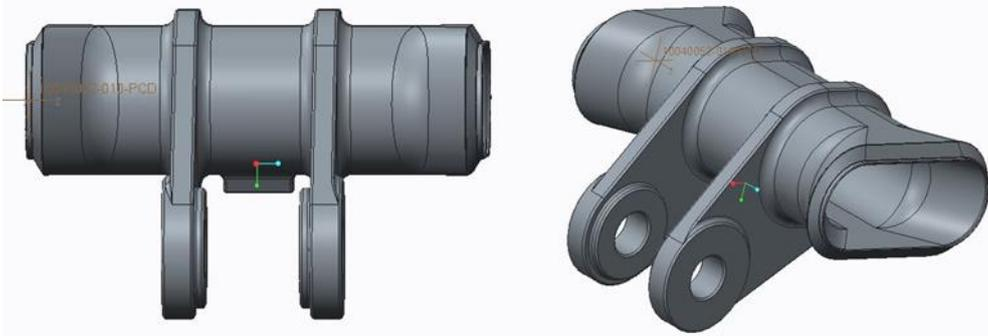
**Figure 1.** Schematic representation of the bearing casting part
