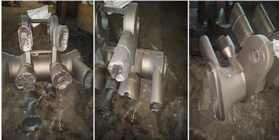
**Figure 7.** The image of poured casting part with the non-filter bottom direct pouring system
