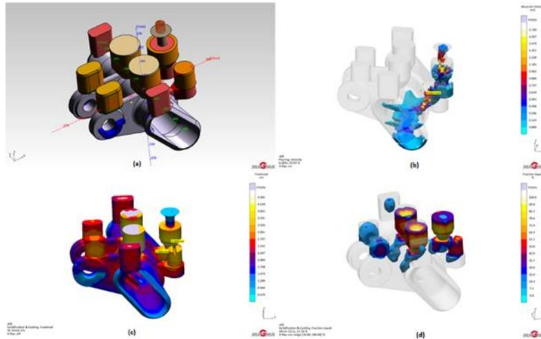
**Figure 4. (a);** The image of the casting part geometry, **(b);** The image of the metal flow and filling simulation of the casting part, **(c);** The image of the feeding mod of the casting part, **(d);** The image of the friction liquid mod of the casting part
