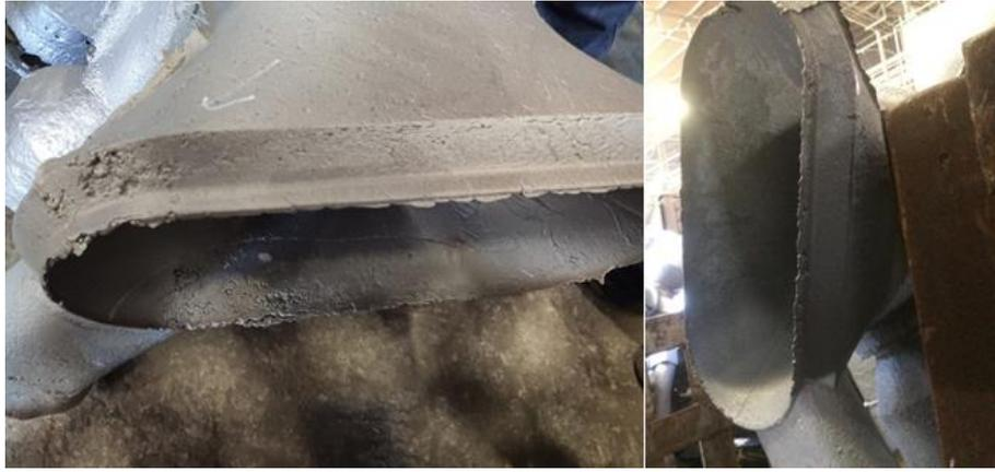
**Figure 3.** The image of poured casting part with the filtered direct pouring system
