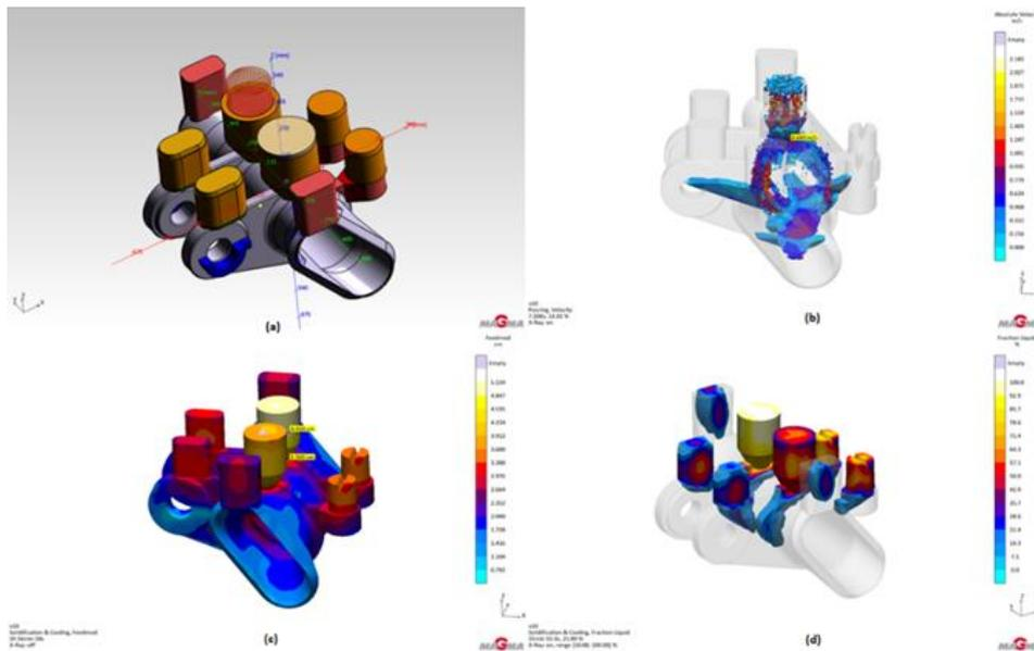
**Figure 2. a);** The image of the casting part geometry, **(b);** The image of the metal flow and filling simulation of the casting part, **(c);** The image of the feeding mod of the casting part, **(d);** The image of the friction liquid mod of the casting part
