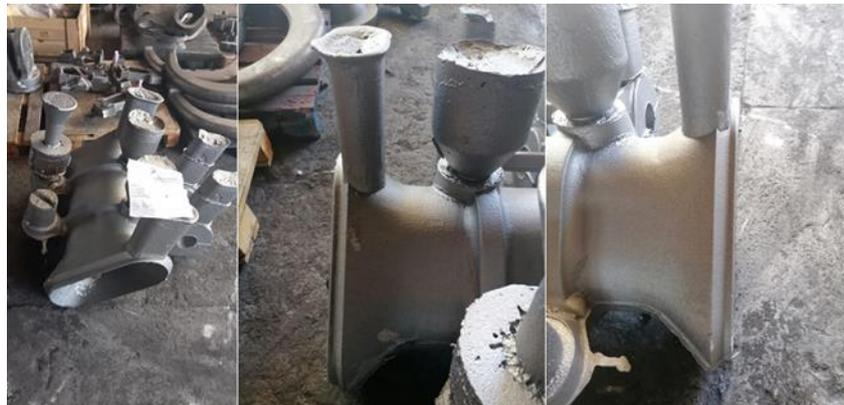
**Figure 5.** The image of poured casting part with the kalpur direct pouring system
