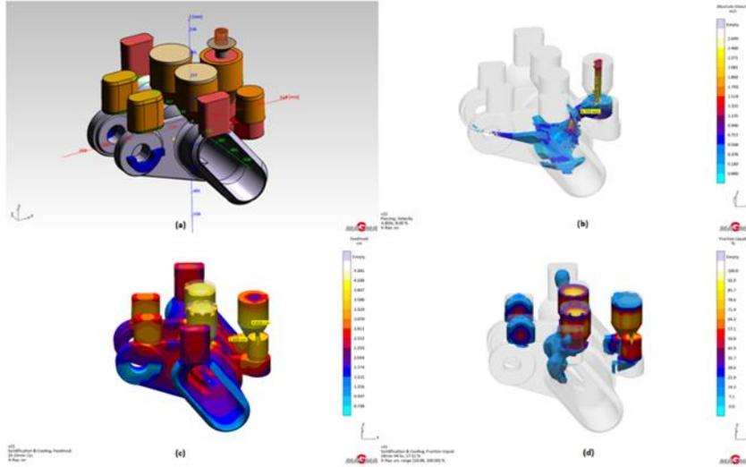
**Figure 6. (a);** The image of the casting part geometry, **(b);** The image of the metal flow and filling simulation of the casting part, **(c);** The image of the feeding mod of the casting part, **(d);** The image of the friction liquid mod of the casting part
