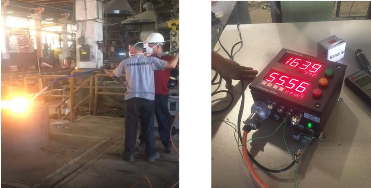
Figure 2. Temperature and oxygen levels measurements in induction furnaces
