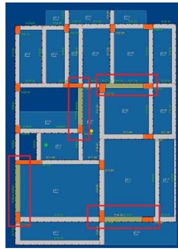
Figure 2. Floor Plan–Reinforcement Curtains
