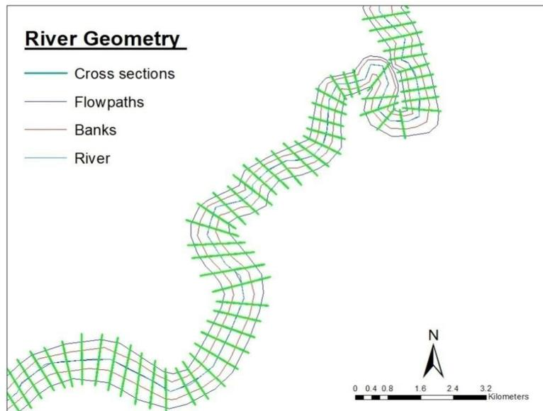
**Figure 3.** Geometry of the selected reach developed in HEC-Geo-RAS
