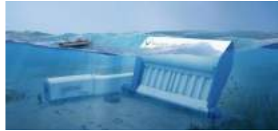
Figure 5: The Oscillating Wave Surge WEC system made by WaveRoller (WaveRoller, accessed 19 Sep 2019)
