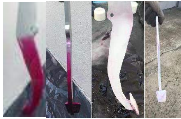
Figure 6: Penetration Test Undestructive Test Pedal
