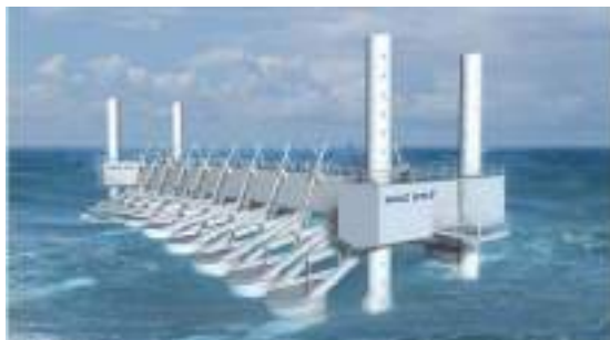
Figure 4: A multi-point absorber system called The Wave Star Machine (wavestarenergy, accessed 19 Sep 2019)
