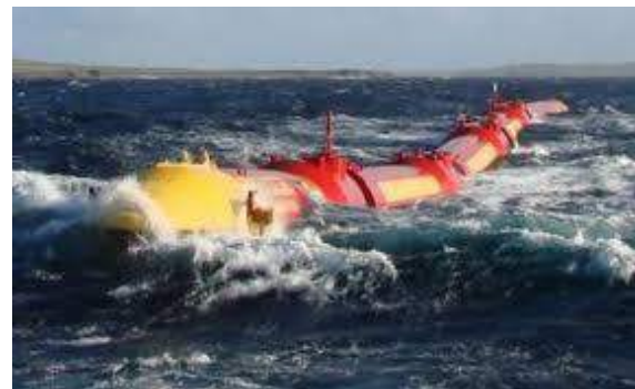
Figure 2: Pelamis Wave Energy Converter system (Solar Thermal, accessed 19 Sep 2019)
