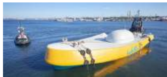
Figure 13: The Penguin Rotating Mass WEC system built by Wello Oy (Wello Oy, accessed 19 Sep 2019)
