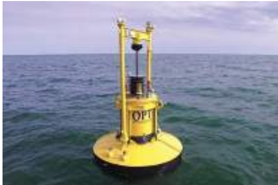
Figure 3: A point absorber WEC system called PowerBuoy (Power, accessed 19 Sep 2019)
