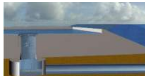
Figure 7: Overtopping system (EMEC, accessed 19 Sep 2019).
