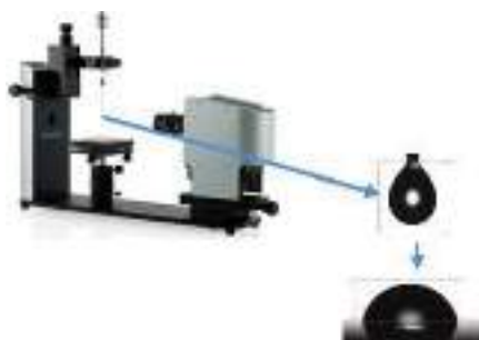
Fig. 8. Attension theta lite device and static droplet method image
