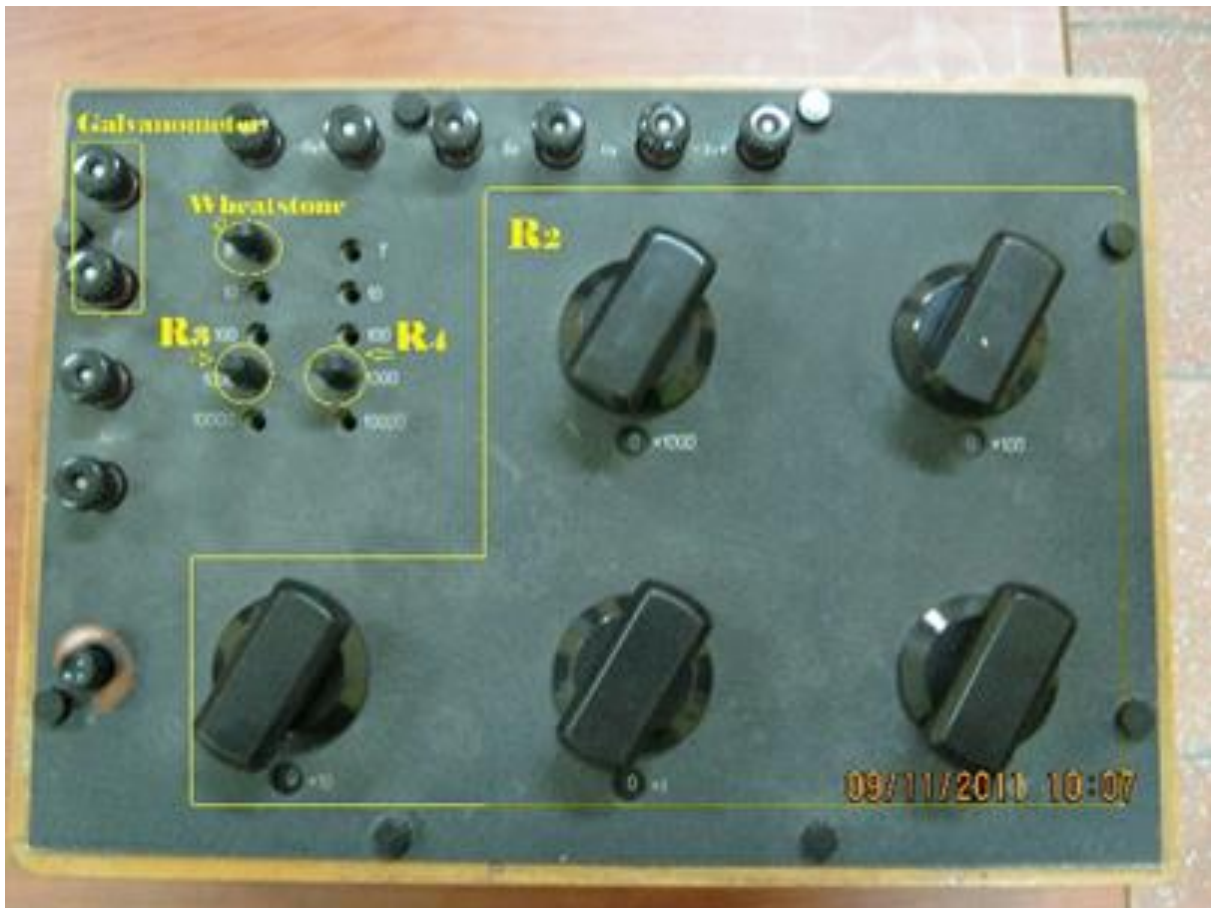
Figure 6. Wheatstone bridge elements used in the MTV Thomson-Wheatstone bridge instrument.
