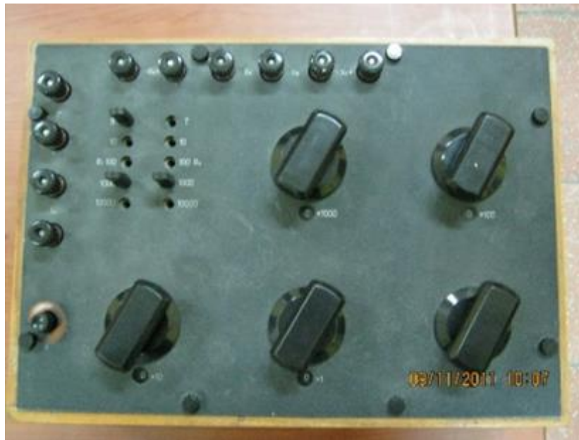
Figure 2. MTV Thomson-Wheatstone Bridge in the Electrical Measurements Laboratory.
