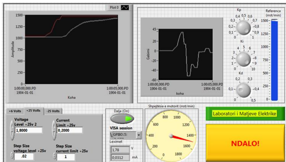
Figure 12. Virtual instrument for DC motor speed control and monitoring front panel.
