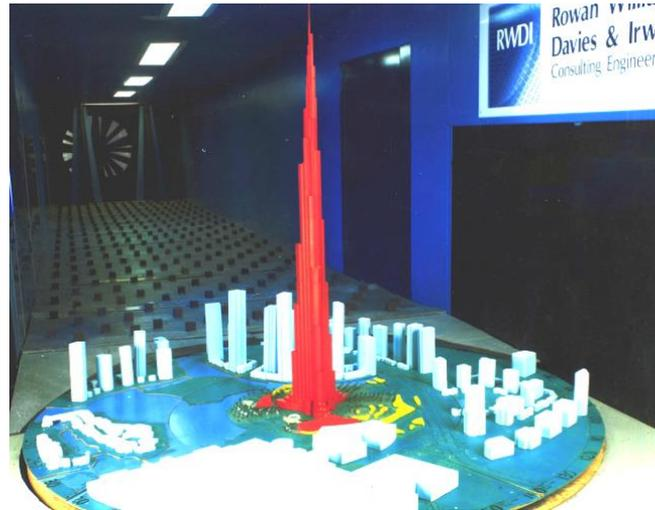
Figure 3. Burj Dubai wind tunnel test [15]
