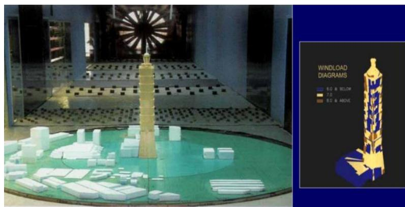
**Figure 2.** Taipei 101 wind tunnel test [14]
