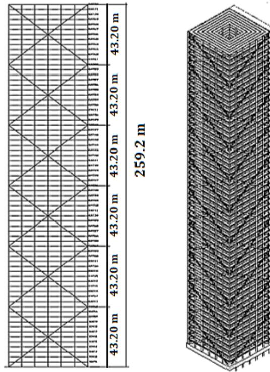
Figure 5. Structural system and three-dimensional view of building model
