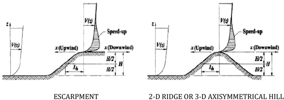
**Figure 6.** Speed increase representation for escarpment and slope [10]
