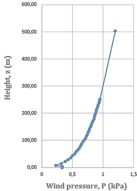
Figure 10: Wind pressure depending on altitude
