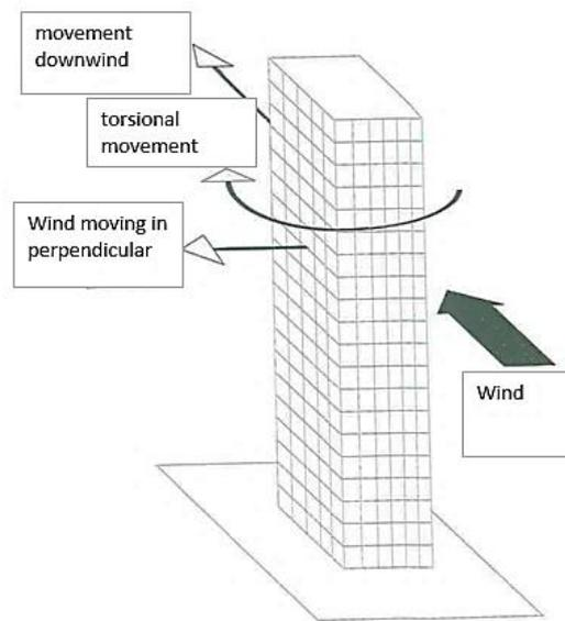
**Figure 1.** Wind-induced building movements [12]
