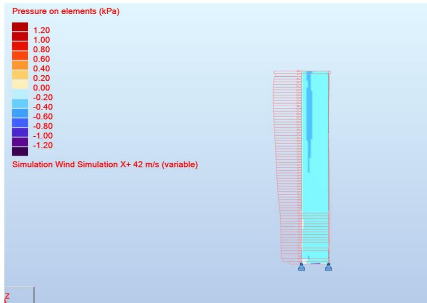
Figure 12: Wind affects on the side surfaces as wind simulation results
