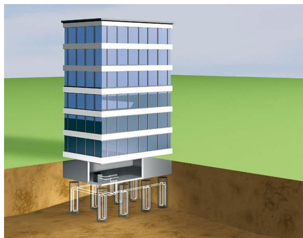
Figure 1. Building with energy piles
