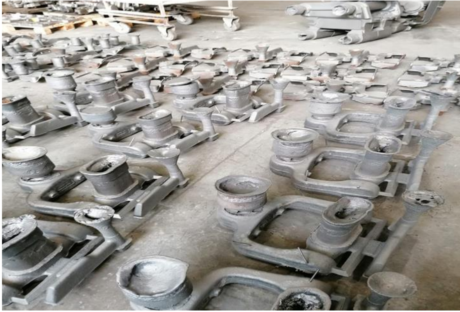
Figure 7. Image of casting parts with a pressurized gating system
