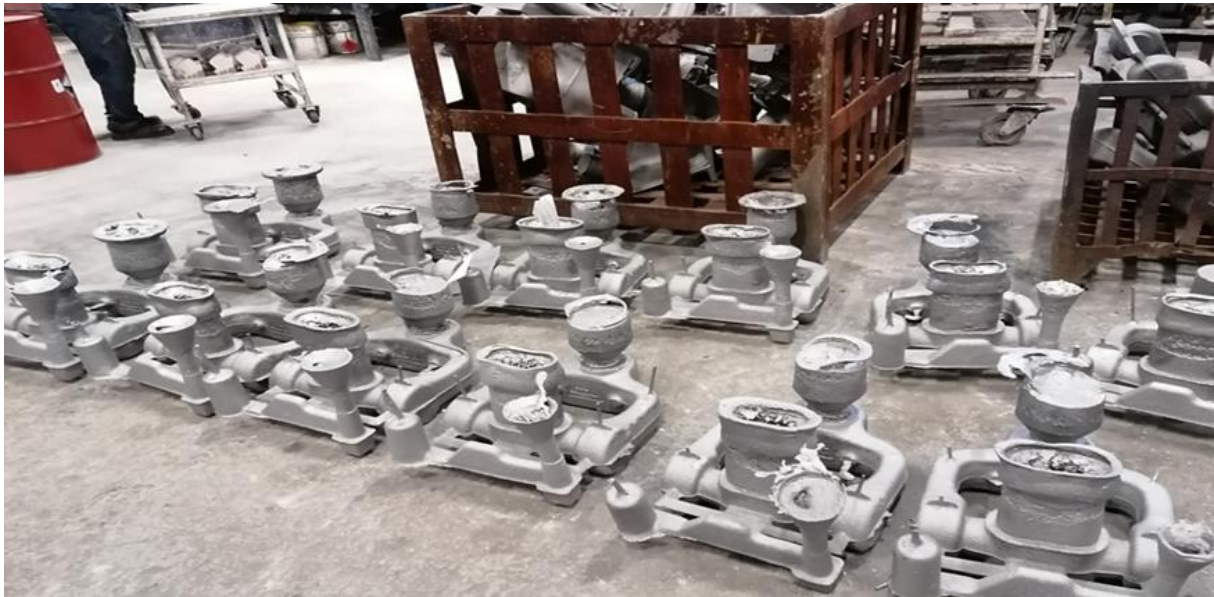
Figure 11. Image of the casting parts with the Spin Trap chamber
