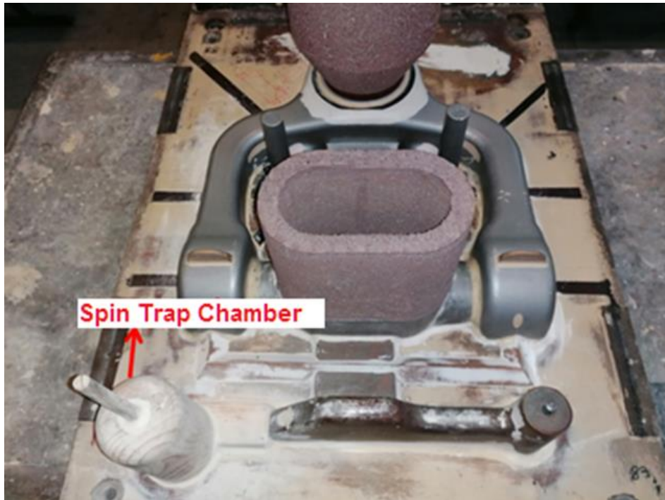
Figure 10. Image of the Spin Trap chamber assembled on the pressurized gating system in the part model
