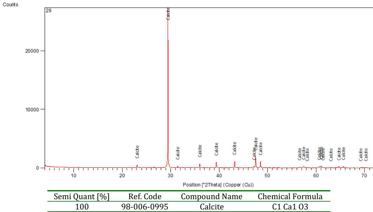
Figure 6. XRD analysis of the calcite sample
