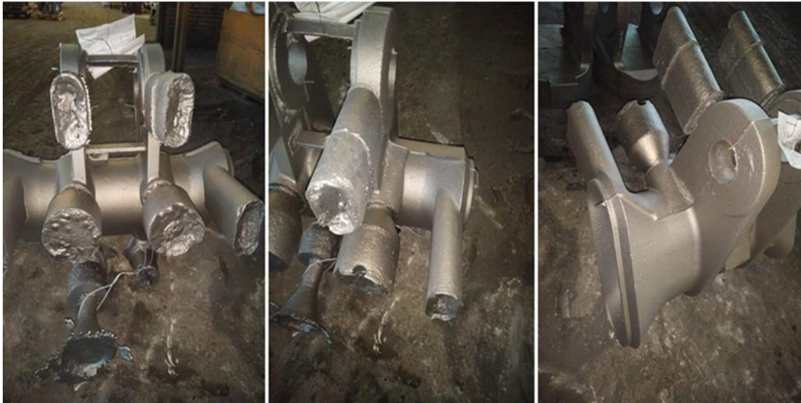
Figure 10. The image of poured casting part with the non-filter bottom direct pouring system
