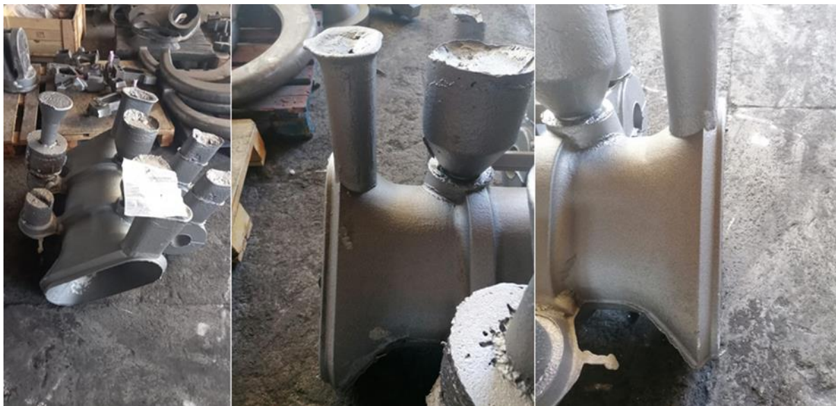
Figure 7. The image of poured casting part with the kalpur direct pouring system
