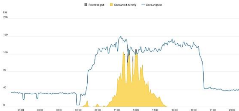
Figure 10. Energy consumed, produced by PV and received from the grid in a factory
