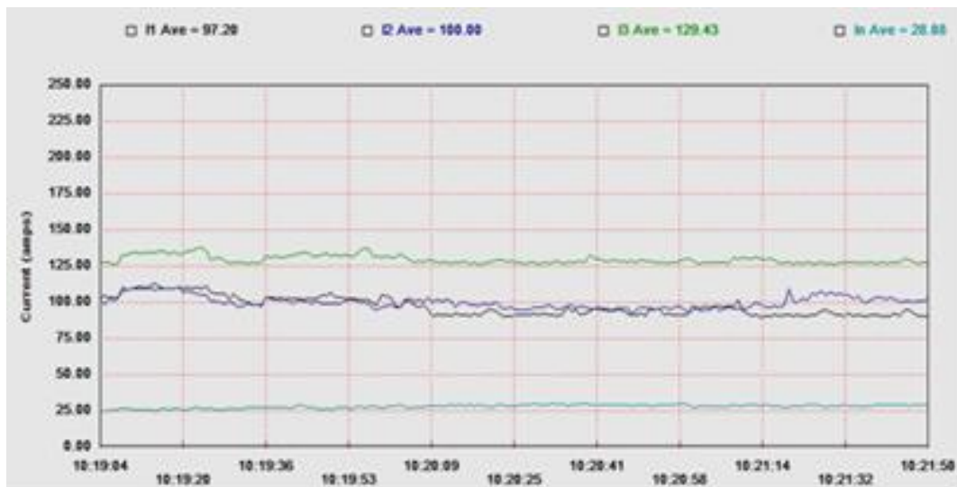
Figure 12. Graph with current amplitudes of the three-phase system
