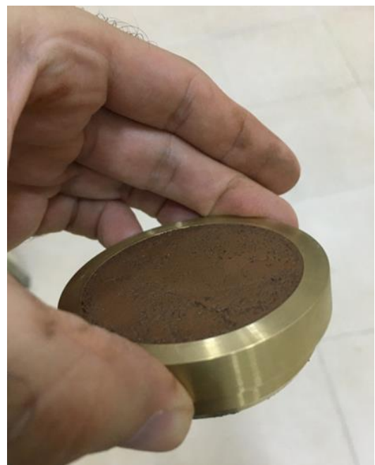
Figure 4b. Soil sample with smoothed surface
