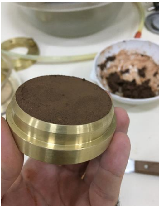
Figure 4a. Soil sample with smoothed surface
