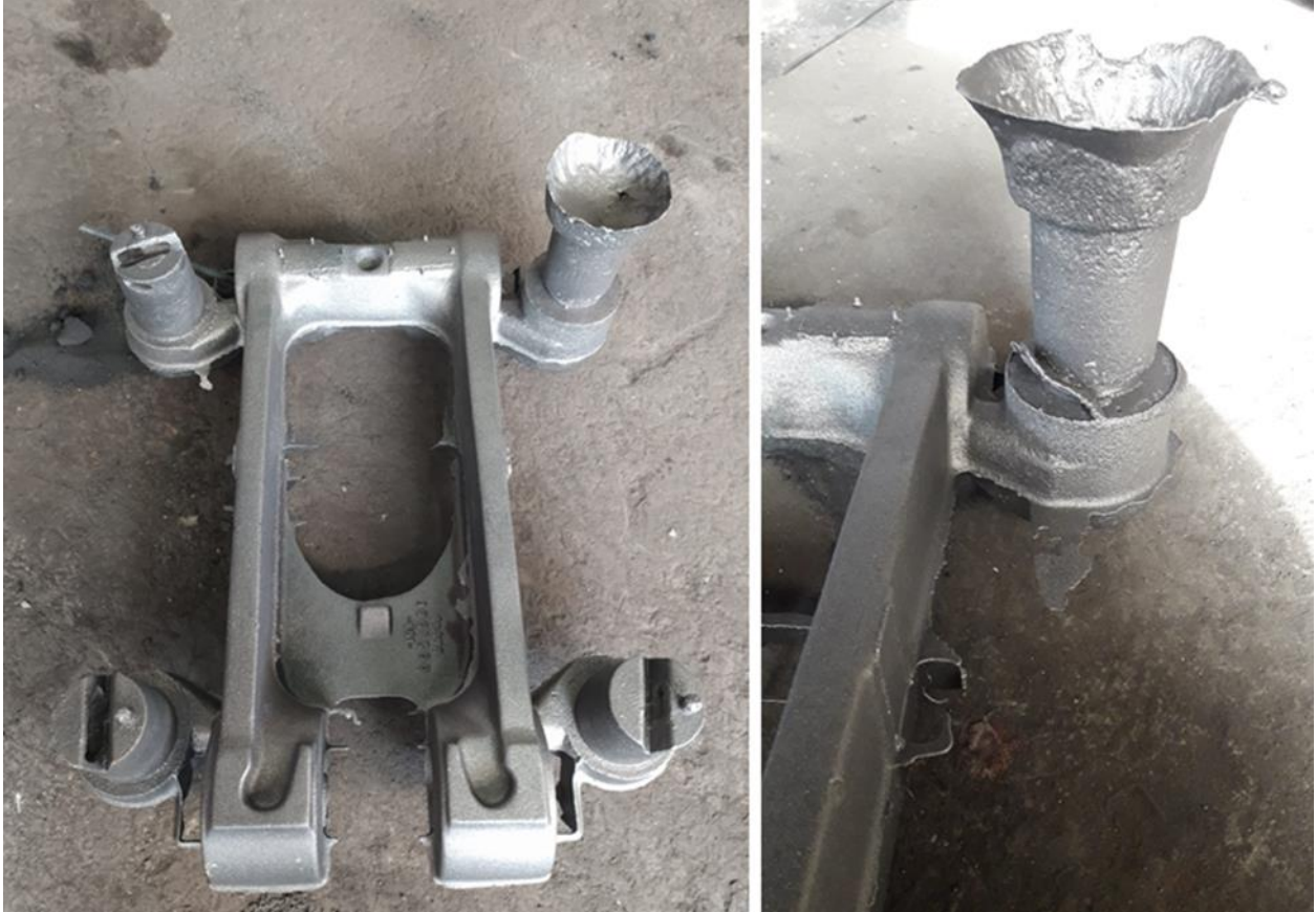
Figure 6. The image of the poured casting part with the kalpur direct pouring system
