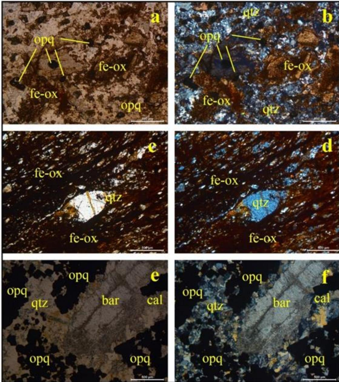
**Figure 4.** Polarizing microscope images of ore zone samples (opq: opaque mineral; fe-ox: iron oxide; qtz: quartz; cal: calcite, bar: barite)
