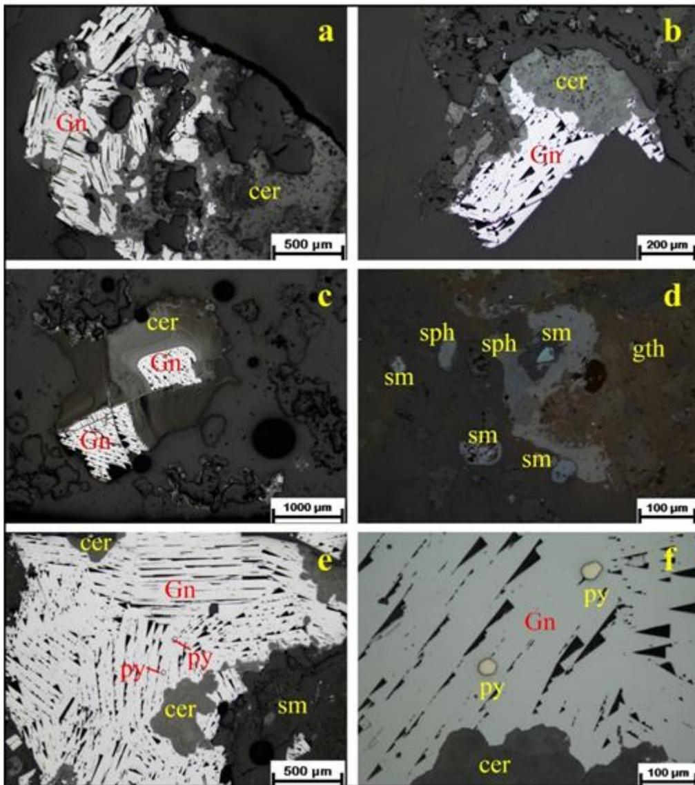
**Figure 5.** Ore microscope views of samples collected from the ore zone (Gn: galenite; cer: cerussite; sph: sphalerite; py: pyrite; sm: smithsonite; gth: goethite).
