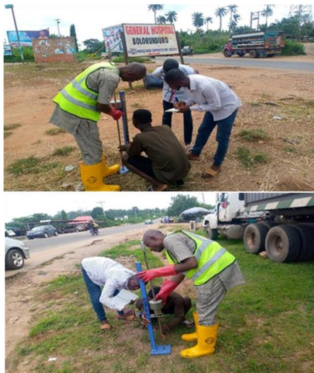
Figure 5. DCPT Field Survey carried out along Akure – Ondo Highway at different locations
