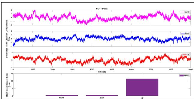
**Figure 4.** Time Series and RMSE of Point Location Components of Network-RTK Solution of N.211.
