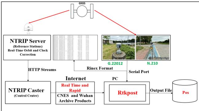
**Figure 2.** Schematic View of The Static-RT-PPP/PP-PPP Methods With a GNSS Receiver/Antenna.
