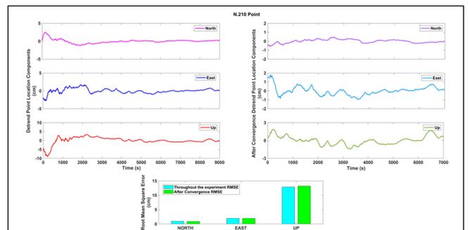
**Figure 5.** Time Series and RMSE of Point Location Components of PP-PPP Solution of N.210.
