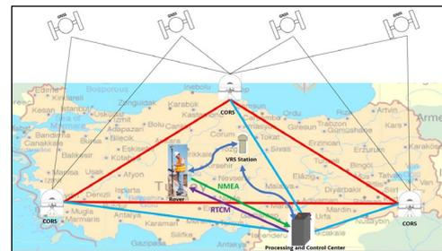
Figure 1. VRS Method in Network-RTK Technique.
