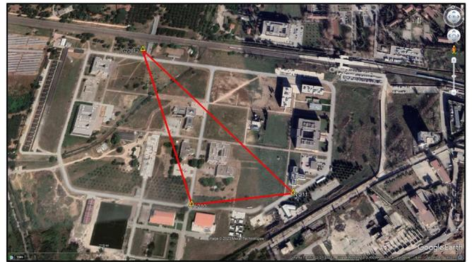
**Figure 3.** Triangulation Stations with GNSS Measurement in The Experiments.
