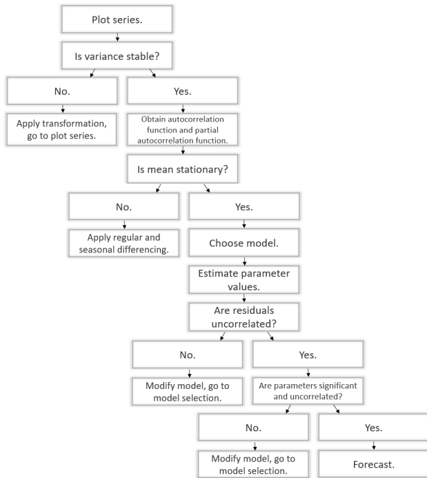
Figure 9. Box-Jenkins forecasting model diagram.
