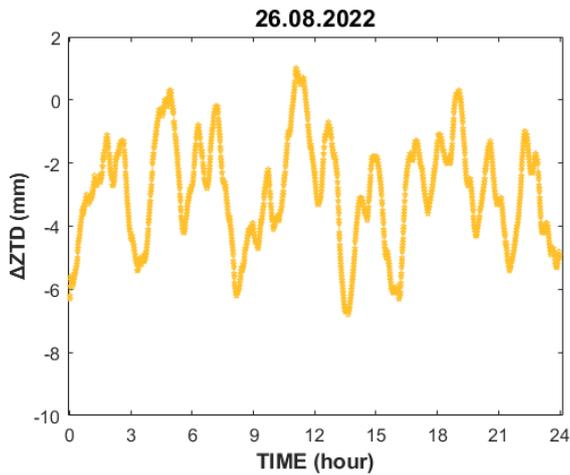
**Figure 3.** ZTD differences between u-blox F9P and geodetic receiver.
