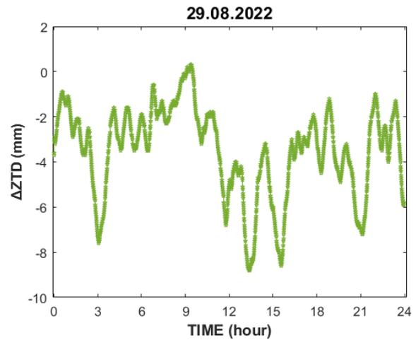
**Figure 6.** ZTD differences between u-blox F9P and geodetic receiver.
