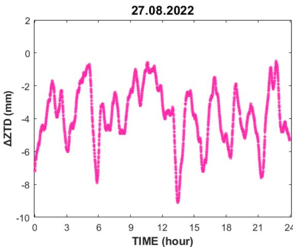
**Figure 4.** ZTD differences between u-blox F9P and geodetic receiver.
