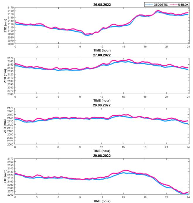
Figure 2. ZTD values of u-blox F9P and geodetic receiver
