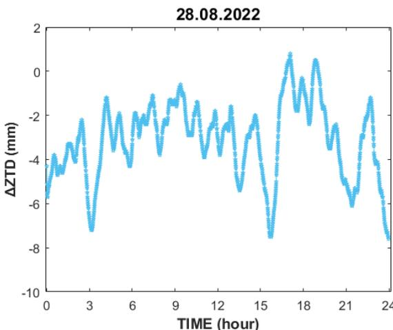
**Figure 5.** ZTD differences between u-blox F9P and geodetic receiver.
