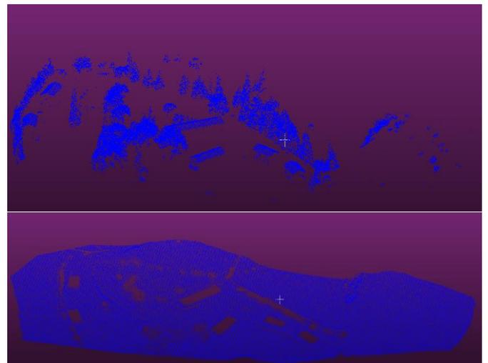
**Figure 2.** The ground (bottom) and the non-ground (top) points of Bergama test area with SMRF
