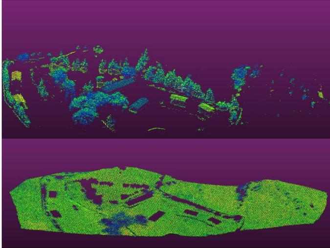
**Figure 3.** The ground (**bottom**) and the non-ground (**top**) points of Bergama test area with CSF
