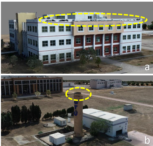
Figure 3. Gaps in the 3D model of a building (a) and a chimney (b)
