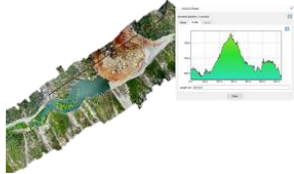
Figure 5. Investigation profile of landslide
