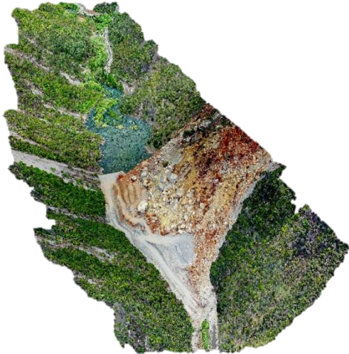
Figure 3. UAV based photogrammetric dense point cloud
