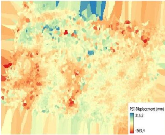
**Figure 5.** Displacement result from PSI - descending mode (mm)
