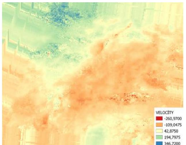
**Figure 4.** Displacement result from SBAS- descending mode (mm)
