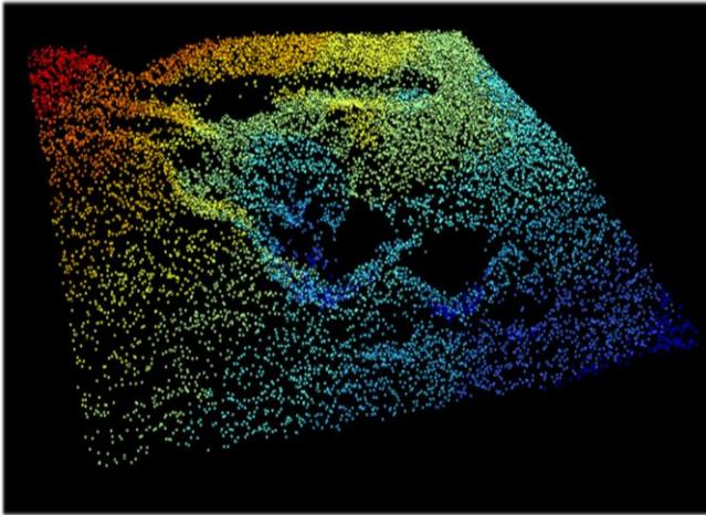
**Figure 9.** Side 3D view of the pothole
