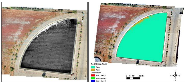
Figure 2. The result of the red/green band ratio (left) and its thematic map (right).
