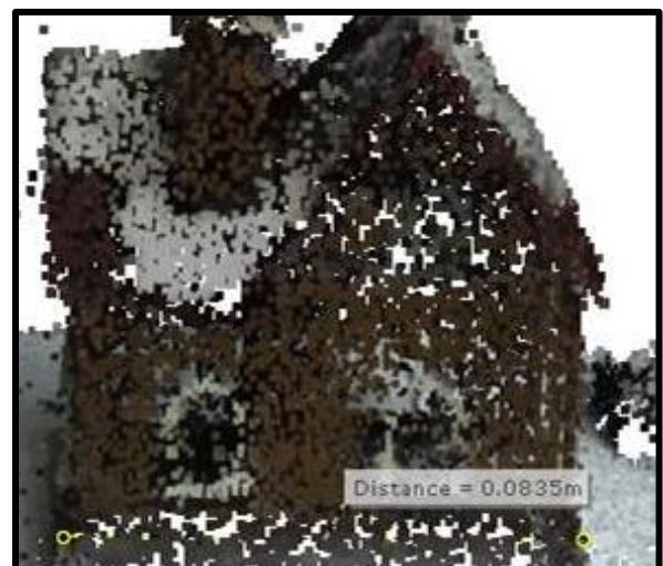
Figure 9. Length measurement of the house figurine obtained by hand-held laser scanning method
