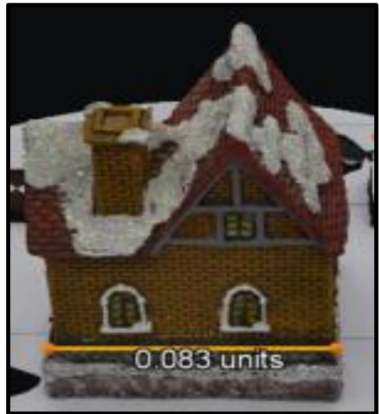
Figure 7. Length measurement of the house figurine obtained by photogrammetric method
