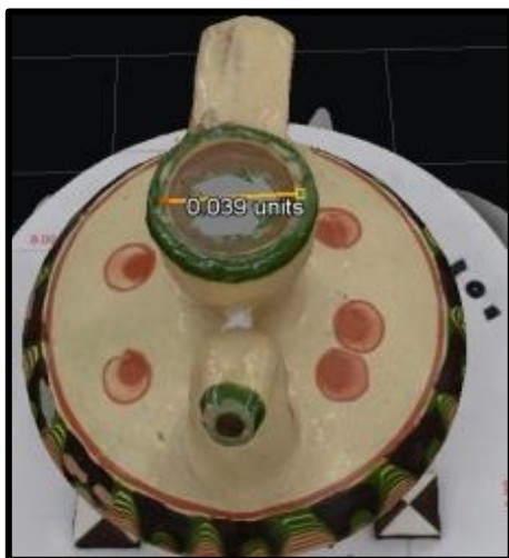
Figure 6. Length measurement obtained from the vase object by photogrammetric method
