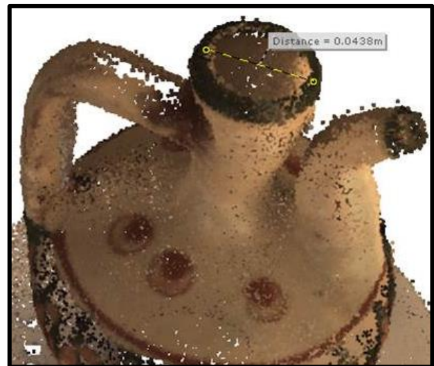
Figure 8. Length measurement obtained from the vase object by hand-held laser scanning method
