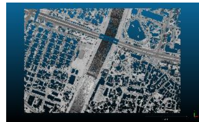
Figure 2. Data Obtained by Leaving the Point Cloud of the Soil Class Alone
