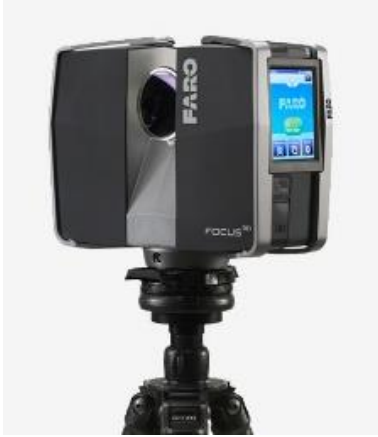
Figure 1. Faro Focus 3D X330 Laser scanner (URL 1)
