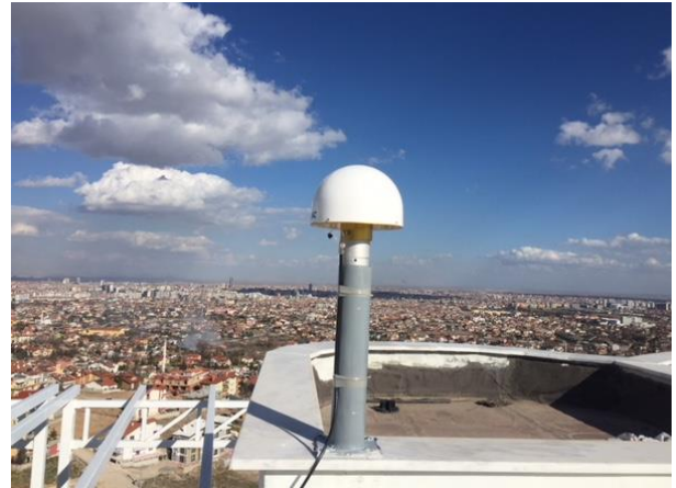
Figure 3. The antenna of NEU-CORS station
