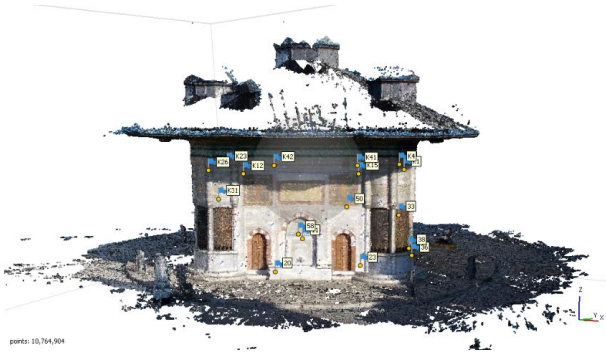
Figure 4. Point cloud produced after close-range photogrammetric survey
