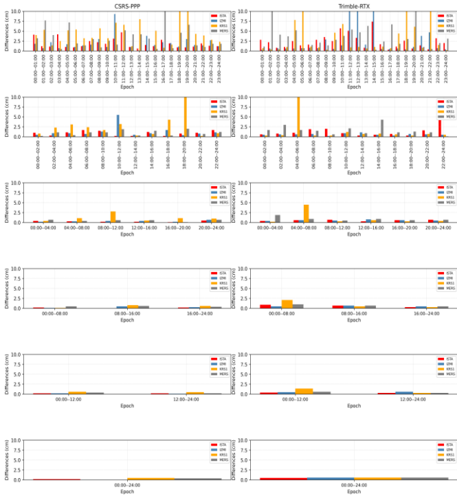
Figure 3. 2D positional differences between known-coordinates and online services for GPS only constellation (left; CSRS-PPP, right: Trimble RTX-PP).
