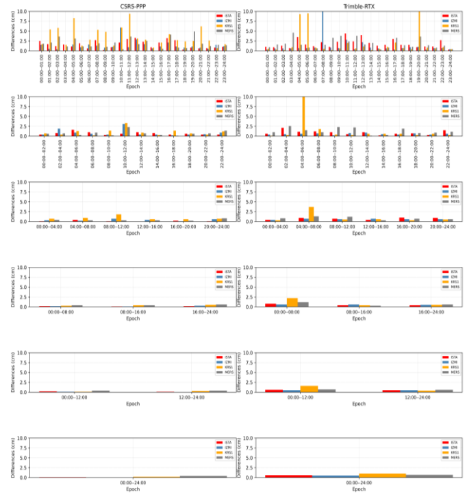
Figure 5. 2D positional differences between known-coordinates and online services for GPS&GLONASS combination (left; CSRS-PPP, right: Trimble RTX-PP).
