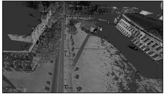
Figure 3. ITU Ayazaga Campus Scanning by Riegl VMX 450 MLS
