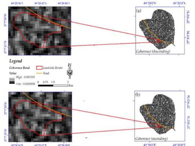
**Figure 4.** Landslide inventory using Sentinel-1 data; (a) descending and (b) ascending
