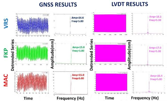
**Figure 2.** Ground motion test: free vibration responses of GNSS (VRS, FKP, MAC) derived time series and FFT spectrum.
