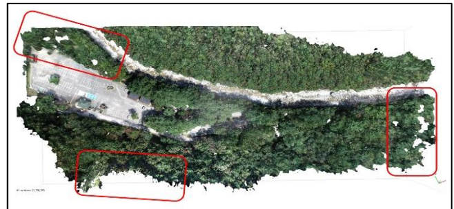
Figure 6. Modeling failure due to lack of image overlap
